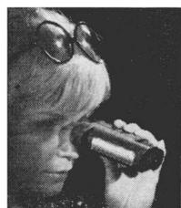
**KODAK Infrared Scope:** A 21-ounce, 1.1X telescope for observing infrared emission or for seeing by infrared illumination. Peak response at 800 nm, 90% of peak at 700-900 nm, total sensitivity range 400 to 1200 nm. Objective can be focused from one foot to infinity. Field of view 26°. Resolves at least 5.5 minutes through focusing eye-
