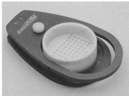
ous samples in a microtitration plate format, then analyze those samples on a large, flat surface. ScreenFast permits close microscopic examination with no possibility of cross-contamination. It is suitable for use with fixed or living eukaryotic cells, virus-containing fluids, DNA precipitates, and bacterial or parasitic suspensions in many applications, including hybridoma and drug screening. Life Technologies. Circle 500.
