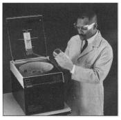
For example, methylene chloride evaporates at a rate up to 9 ml per minute per tube. The vortex motion creates a rinsing action that helps keep analytes in solution so excellent recoveries are achieved. Sensors automatically detect when endpoint has been reached. Labconco. Circle 140.
