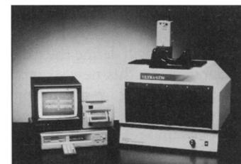
tographed images on a 3.5-inch floppy disk and provides for serializing and dating of the stored images. The PHD 2000 can also enhance the images with integration to intensify the faint bands and averaging to reduce the background noise. **Ultra-Lum. Circle 146.**
