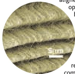
aligned carbon nanotubes that behave as open-cell flexible foams. The films can be reversibly squeezed to only 15% of their original thickness without structural failure, despite the significant zigzag bucking of the nanotubes. The nanotubes act as elastic compression springs; they are highly compressible along their axis but regain most of their free length after a compressive load is released.
