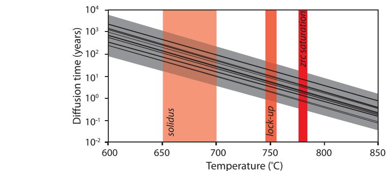
**Fig. 2. Diffusion durations as a function of temperature, calculated for all measured peaks.**
