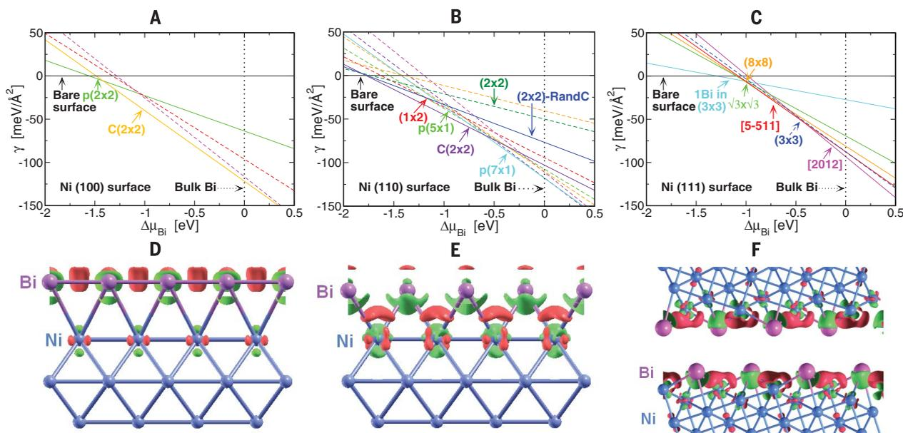
**Fig. 2. Results of DFT calculations for Ni-Bi free surfaces and a grain boundary.** (A to C) DFT calculations of surface free energy as a function of chemical potential for various Bi-based superstructures on three different Ni surfaces: (A) Ni(100) surface, (B) Ni(110) surface, and (C) Ni(111) surface. (D to
