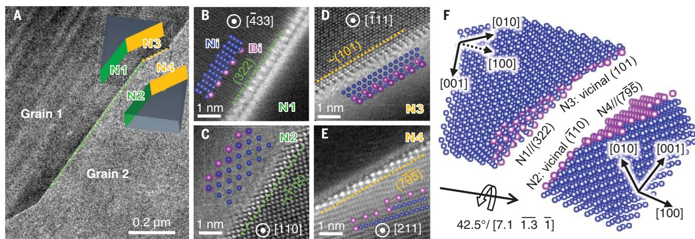
**Fig. 3. Grain boundary facets in Bi-doped Ni.** (A) HAADF-STEM image of a general grain boundary in Bi-doped Ni, which contains micrometer-sized facets. The grain boundary plane pairs ("grain boundary surfaces") of one facet are marked as N1 and N2 (green) and those of a second facet are marked as N3 and N4 (yellow). (B to E) HAADF-STEM images of the four grain boundary facet planes (with inset atomic diagrams) showing
