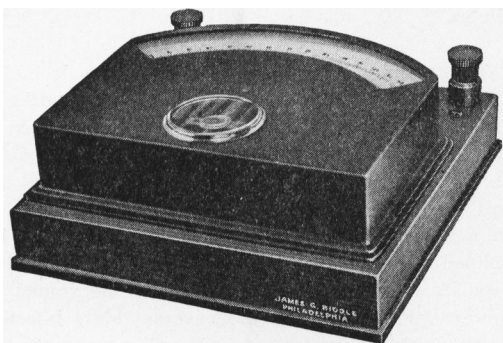
Cat. No. 560001 Precision 10-ohm Millivoltmeter. 45 millivolts drop for full scale deflection. 150 scale divisions. Supplied with a third terminal for a range of 3 volts, resistance 1000 ohms.
