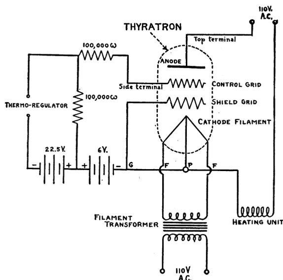
FIG. 1. Wiring diagram for thyratron control for incubators and water-baths.
