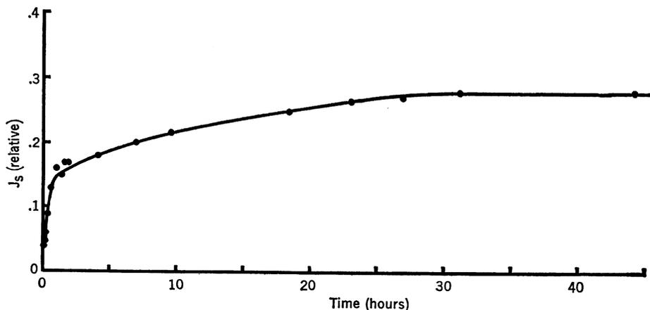
Fig. 3. Saturation magnetization as a function of heating time at 400°C for a powdered sample heated in the Curie balance.
