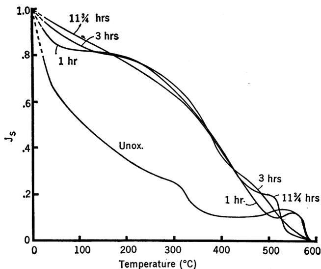
Fig. 1 (above). Curves of saturation magnetization ( $J_s$ ) plotted against temperature for an unoxidized sample and for samples held at 400°C for 1, 3, and 11¼ hours before measurement.
