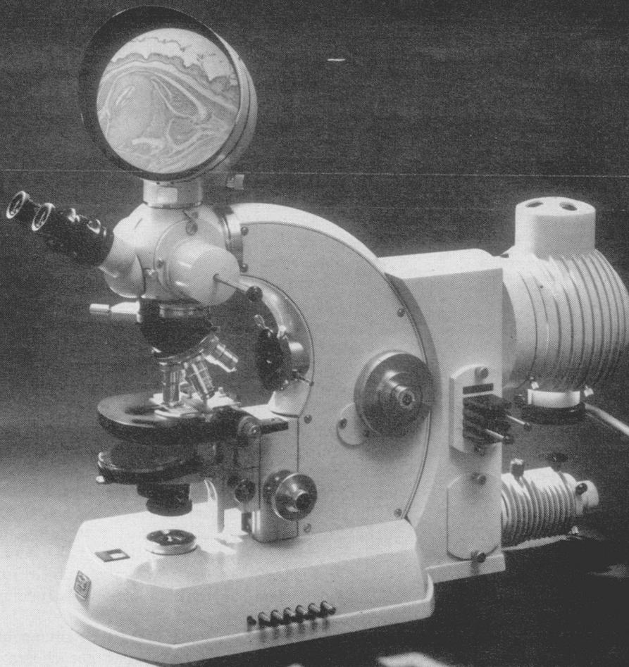
The Zeiss Photomicroscope II equipped with optional viewing screen.
