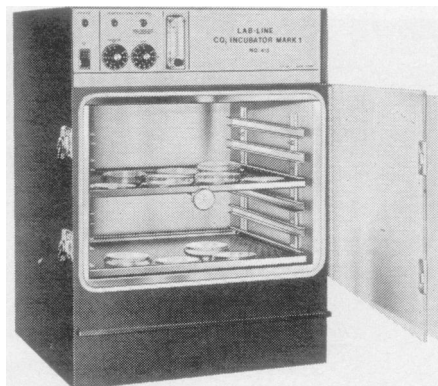
Fig. 3. The Mark I carbon dioxide incubator from Lab-Line provides 4 square feet of shelf space (with two shelves).
