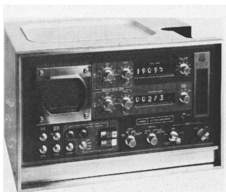
Fig. 1. The model 4800A Cytofluorograf measures light scattering and fluorescence. Cells may be studied with fluorescent techniques such as the Schiff procedure for DNA, with vital stains such as acridine orange for viability, or with fluorescein compounds to characterize cellular enzymes in addition to automatic sizing and counting.
