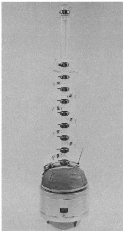
for each application. System comprises eight bubble cap sections, eight sampling units, a liquid divider, a coaxial condenser, a boiling flask, product receiver, heating mantle, framework, and clamps. Systems are available in several diameters. Kontes. Circle 837.
