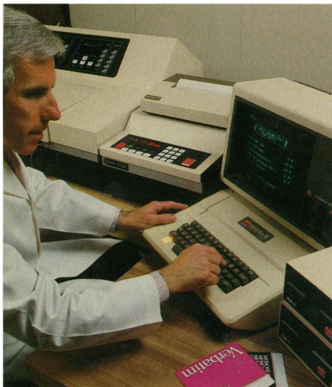
The new Varian DMS 90-PLUS Kinetics System adds the Programmable Cell Changer to the spectrophotometer system — together they form a powerful and completely automatic reaction rate system for enzyme assays.
