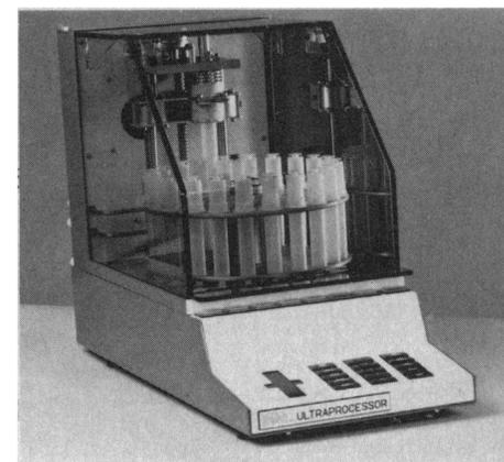
and sealed reagent vials. Specimens are moved from vial to vial without cross-contamination. The 3189 Ultraprocessor accommodates all specimens embedded in resin, whether destined for light or electron microscopy. RMC. Circle 550.
