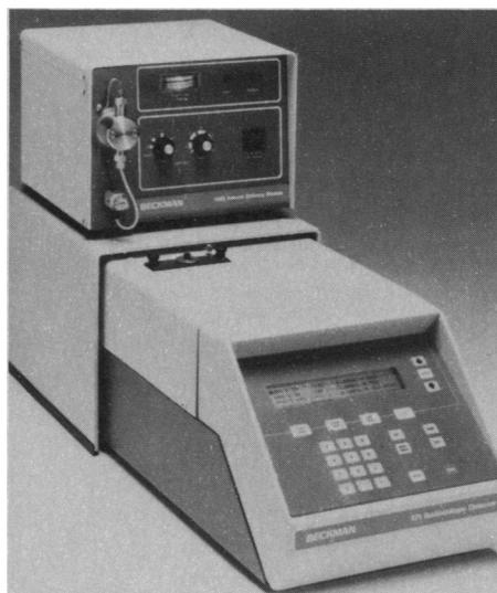
easy decontamination. Self-adjusting circuitry optimizes counting conditions for packed cells or liquid cells. Other features include a four-line, 40-character, liquid crystal display, menu-driven programming, automatic fraction-collector control, luminescence correction, automatic background subtract, automatic start and stop, and user-accessed diagnostics. Beckman Instruments, Nuclear Systems Operations. Circle 525.
