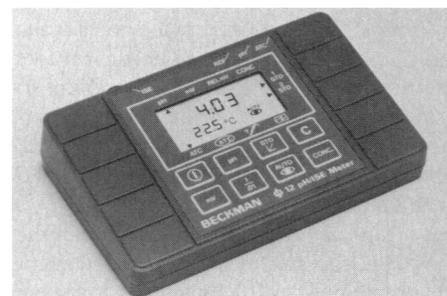
tion or calibration. Only when the measurement approaches stability is it displayed and locked. The meter has a resolution selector of 0.1 or 0.01 for *pH*. Beckman Instruments, Scientific Instruments Division. Circle 622.
