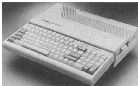
play 64 colors (16 at once) with high-resolution graphics of 640 by 350 pixels. Also built in is a clock with a rechargeable battery. The computer has one 5.25-inch disk drive and an interface for a second. Other interfaces include a parallel printer port, a RS-232 serial port, and a joystick port. Video Technology Computers. Circle 620.
