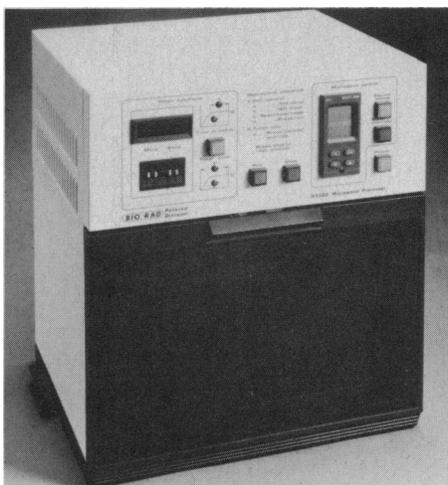
processing procedures. The processor has a programmable temperature control, a timer, and an elapsed-time light-emitting diode display. A probe monitors and controls solution temperatures. Temperature can be controlled within 1°C, and time, within 1 sec. Bio-Rad Polaron Division. Circle 657.
