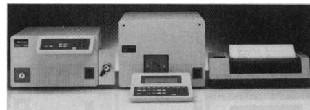
Pump and the LC-135 dual-channel detector. Shallow gradients under the low flow rate conditions typically used in peptide mapping are not a limitation with the system. The LC-135 detector provides dual-channel detection for monitoring both peptide bonds and aromatic residues. The system is capable of routine peptide mapping at the 5- to 10-pmol level and is compatible with high-speed and narrow-bore peptide columns. Perkin-Elmer. Circle 574.
