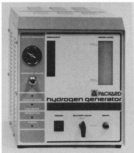
ometer mounted on the generator's front panel. The Model 8200 uses an exclusive electrochemical process to extract hydrogen from deionized distilled water. The hydrogen is then filtered and dried before delivery to a standard plumbing output port on the back of the unit. Packard Instrument Co. Circle 531.
