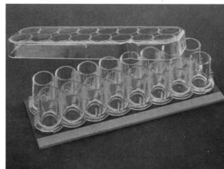
user to take advantage of multichannel pipettes and other devices designed for use with 96-well plates. The 16 Well has two rows of eight wells, each well with a volume of approximately 0.3 ml and a growth surface of 0.32 cm<sup>2</sup>. Each unit has a unidirectional lid with condensation control rings. Nunc. Circle 455.
