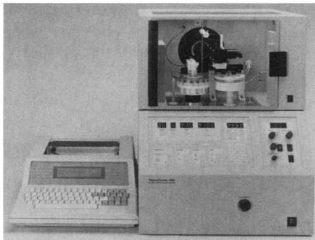
compatible with Waters data workstations and features a high-sensitivity, low-noise ultraviolet/visible detector designed to detect even trace level components. The system offers both automatic hydrostatic and electromigration injection for application flexibility. Waters, Division of Millipore. Circle 439.
