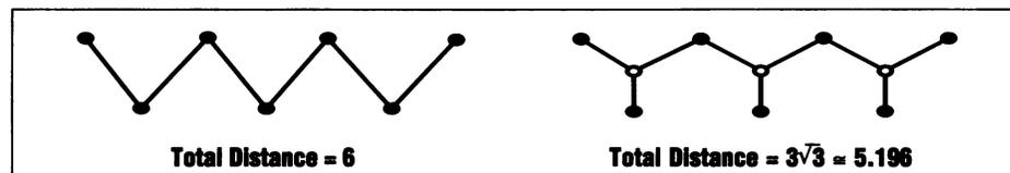
**Networking.** A "shortest" network (left) can be shortened by introducing extra points (right). The savings shown here—13%—is the maximum possible.
