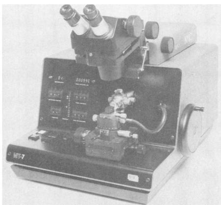
increments. With a powerful driven cutting stroke and microprocessor-controlled mechanical specimen advance, the MT-7 makes light work of sectioning ceramics, superconductors, metal oxides, bone, teeth, and composite materials. The MT-7 features high-quality stereozoom optics, multifunction adjustable lighting, a swivelling and tilting stereomicroscope, a digital section counter, and built-in vibration isolation. Research and Manufacturing Co. Circle 480.
