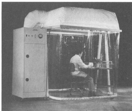
formly through a unique, clear perforated ceiling. The plenum is attached to collapsible "Gull Wing Ceilings," which fold down to allow the device to pass through a standard 36-inch doorway, then expand to allow 40 square feet of inside space. Entry and exit is through clear vinyl curtains, which also serve as a barrier from the outside. The room takes less than 30 min to set up. Airo Clean Engineering. Circle 457.
