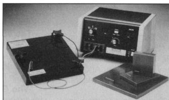
electrophoresis gels and hybridization membranes are sandwiched horizontally between layers of filter paper soaked in an electrode solution. Multiple gels can be processed by "stacking" the sandwiches. Electrodes are in direct contact with the sandwich, creating a homogeneous electric field that ensures even transfer. Fisher Scientific. **Circle 92.**
