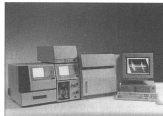
user-oriented format that is simpler, more compact, and more economical than any mass spectrometer adapted for HPLC work, according to the manufacturer. The mass detector provides library searchable mass spectra for identification of up to 1000 atomic mass units. **Millipore. Circle 144.**
