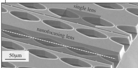
Micrograph showing an array of x-ray lenses fabricated in diamond.
