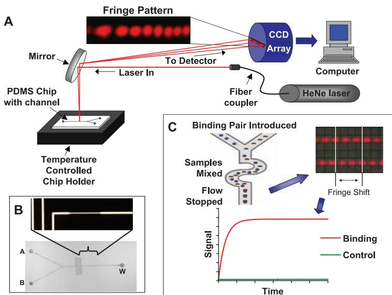
**Fig. 1.** (A) Experimental setup for BSI. (B) Microfluidic chip with serpentine mixer and restriction. (C) Photograph of representative fringe patterns showing a RI-induced position shift of the fringes, a representation of a binding event, and observed signal for a control and reactive pair binding event.
