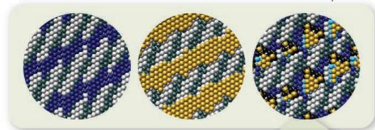
tials (extra atoms stuffed between lattice sites). Demkowicz *et al.* use simulations to probe the effects of adding or removing atoms in copper-niobium multilayer nanocomposites. Two flaw-free interfaces can form between the Cu and Nb. The first occurs from the joining of the face-
