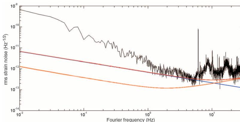
**Fig. 1.** Strain noise measured by the FBG resonator in (3). The blue line is the noise calculated from Duan’s model (12), the orange line is the comb-stabilized strain noise, and the red line is the RMS sum of them.
