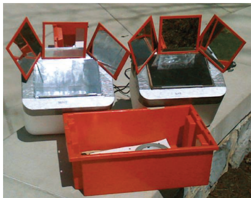
Solar ovens constructed by students. The black one reaches a higher temperature. Both were capable of baking cookies.
