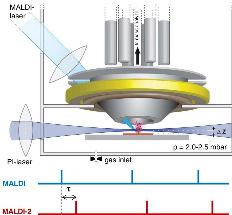
**Fig. 1. MALDI-2 ion source.** Schematic drawing of the modified MALDI ion source of the Synapt G2-S mass spectrometer with primary MALDI and PI laser beams and shielding aperture for increasing the cooling gas pressure in the region of ion generation; 2.0 to 2.5 mbar of N<sub>2</sub> were used for the MALDI-2-MSI measurements. The lower panel illustrates the laser pulse triggering sequence.
