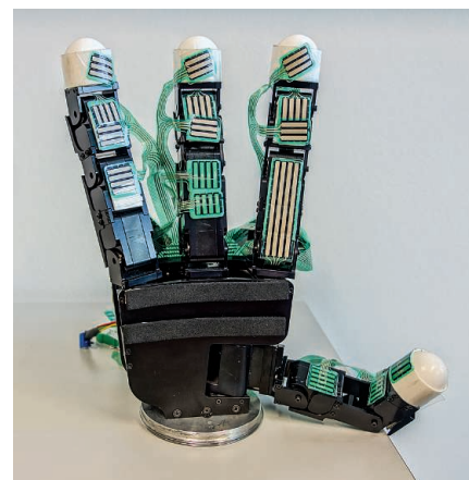
Strategically placed tactile sensors help a robotic hand grasp unknown objects while maintaining low contact forces.
