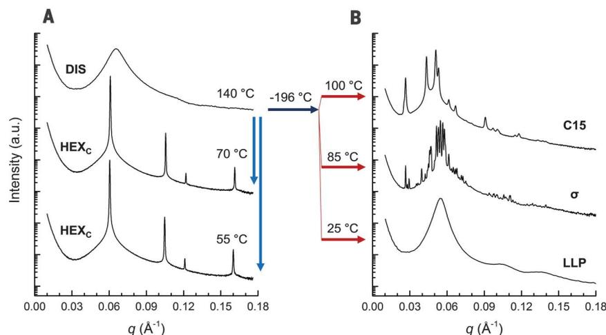
**Fig. 4.** SAXS patterns obtained from IL-52-20 after different thermal treatments. (A and B) Data were obtained using the same procedures identified in Fig. 3, where  $T_{\text{ODT}} = 132^\circ\text{C}$  for the  $\text{HEX}_c$  to DIS transition. The data are vertically shifted for clarity.
