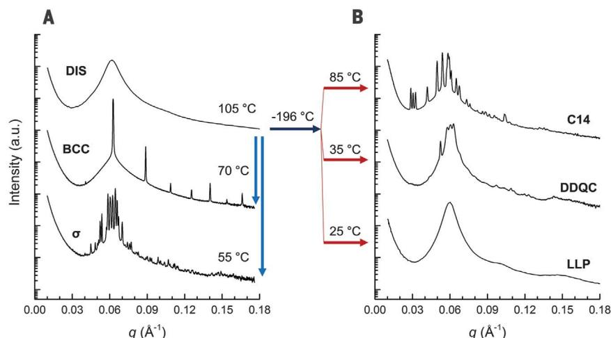
**Fig. 3.** SAXS patterns obtained from IL-58-15 after different thermal treatments. (A) Direct cooling from the disordered (DIS) state, where  $T_{\text{ODT}} = 99^\circ\text{C}$  for the bcc to DIS transition, and (B) after immersion in liquid nitrogen and reheating. The data are vertically shifted for clarity.
