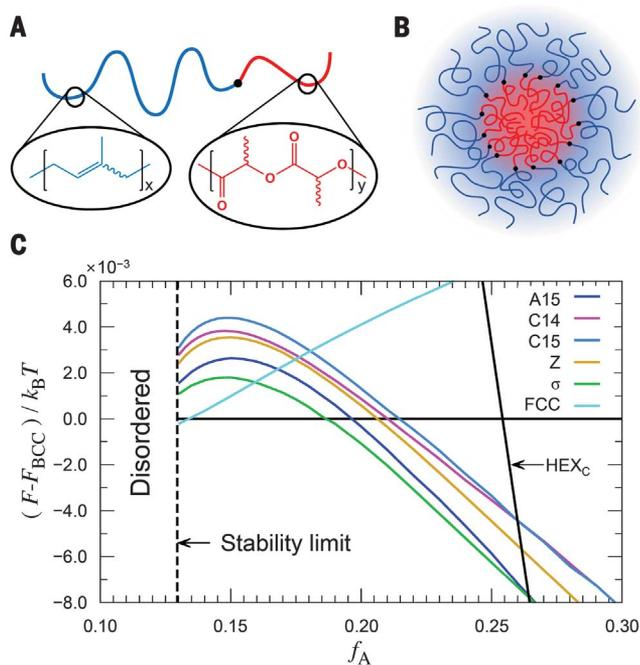
**Fig. 1. SCFT free-energy calculation of asymmetric diblock copolymers.** (A and B) Schematic representation of (A) AB diblock copolymer [(Inset) Chemical structures of PI and PLA blocks] and (B) a micelle particle formed by the polymer chains. (C) SCFT free-energy difference between various Frank-Kasper phases with respect to bcc as a function of  $f_A$  for  $\chi N = 40$  and  $b_A/b_B = 2$ . See figs. S2 and S3 and table S1 for additional calculations.
