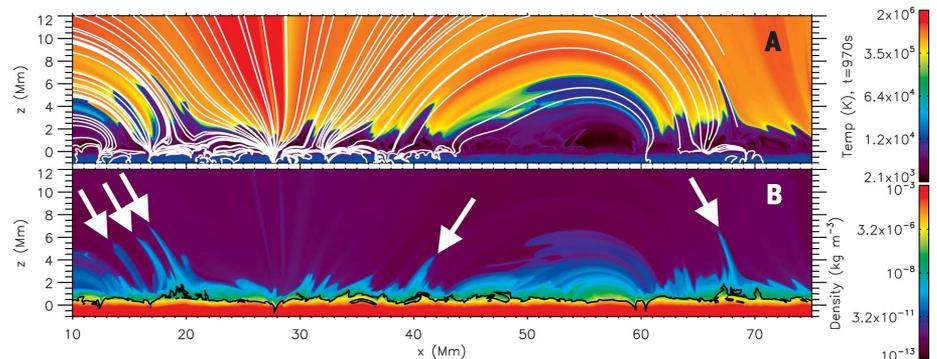
**Fig. 1. Spicule-like features (indicated by arrows) occur in our radiative MHD simulations.** They appear as dense, cool intrusions in the hot corona, originating from the boundaries of the strong magnetic regions. (A) Temperature and (B) density maps are shown on a logarithmic color map with white magnetic field lines (A) and black contours where plasma  $\beta = 1$  (B). *t*, time.
