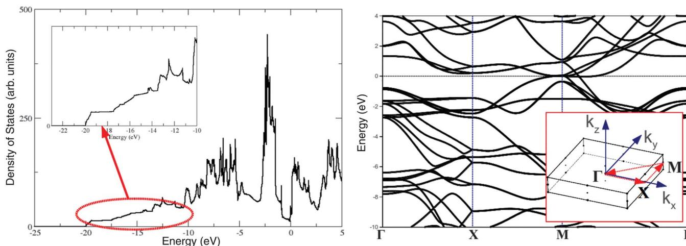
**Fig. 4. Band structure and electronic densities of state of FeH<sub>5</sub> at 147 GPa.** (Left) Electronic density of states of FeH<sub>5</sub>. (Right) Electronic band structure plotted on a path in the  $k_z = 0$  plane. (Inset) View of
