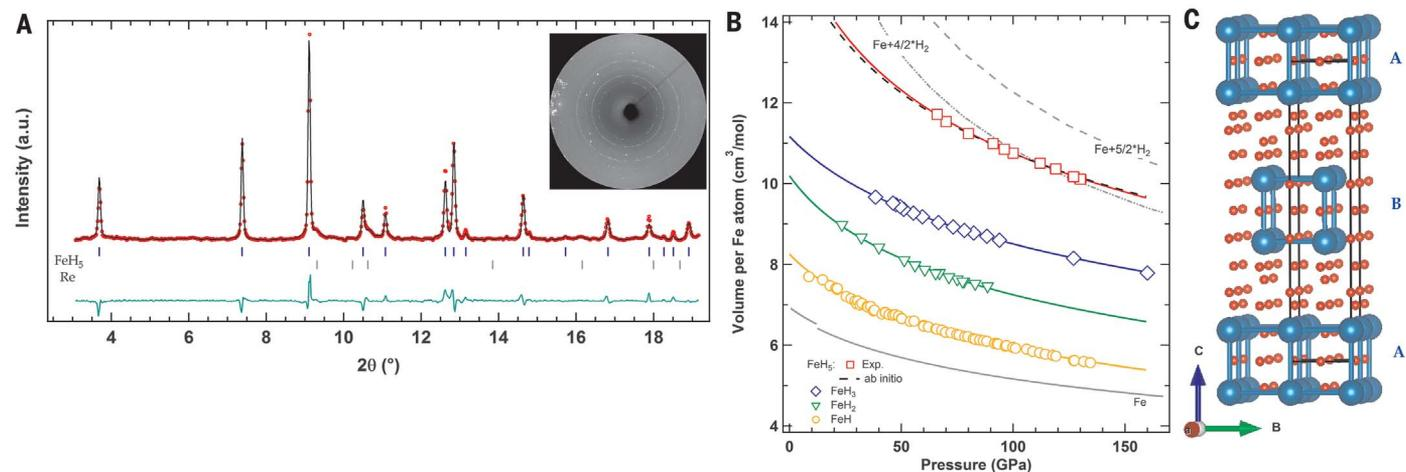
**Fig. 1. Equation of state and structure determination of FeH<sub>5</sub>.**
