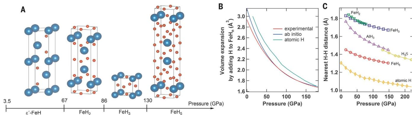
**Fig. 2. Hydrogen in the host lattice.** (A) Evolution of the stoichiometry and of the structures of iron hydrides synthesized in excess of hydrogen as the pressure increases. (B) Volume expansion by adding one H to FeH<sub>*n*</sub>, compared to the equation of state of pure atomic hydrogen. The volume
