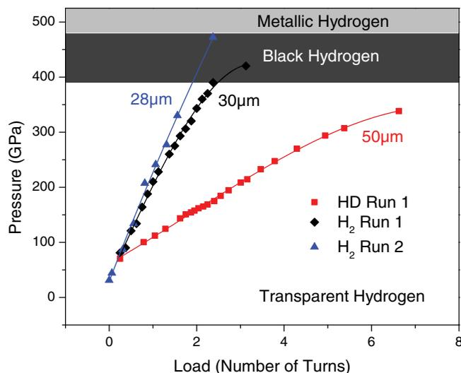
**Fig. 1.** Load curves for our diamond anvil cell for three runs with the same DAC but different diamond culet flat diameters. The blue triangles are for the MH run.
