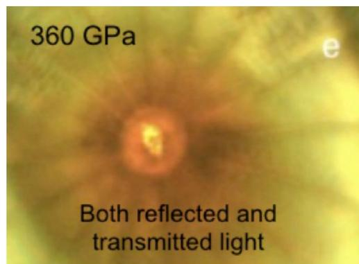
**Fig. 2.** Photo of a sample of hydrogen in transmitted and reflected light at 360 GPa and a temperature of 80 K.
