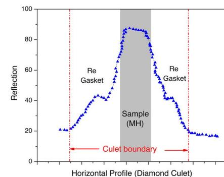
**Fig. 2. Reflectance of the gasket and MH across a culet diameter.**
