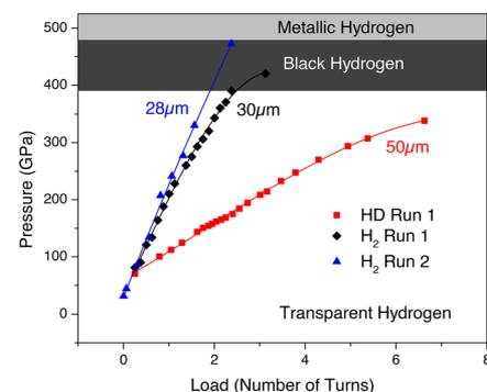
**Fig. 1. The load versus pressure for three different runs with our DAC.** The data points are measured pressures. The curves show plateauing at the highest loads, but the curve in which MH was made has not yet plateaued, indicating that higher pressures were accessible. The culet diameters are indicated for each curve.
