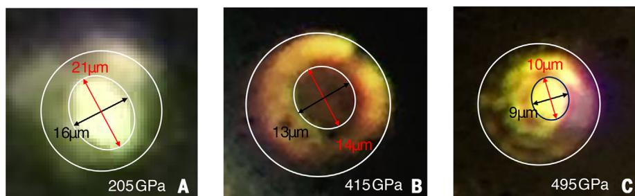
**Fig. 4. iPhone photos and the sample dimensions.** In (B) and (C), we can use the known dimension of the diamond culet to set the scale. The culet is observable and has no important change in dimension with increasing pressure. The culet is not clearly observable in (A) because the sample was back illuminated. In (A), we estimate the dimensions from knowledge of the starting dimensions of the gasket hole; this has a larger uncertainty of a few  $\mu\text{m}$ .
