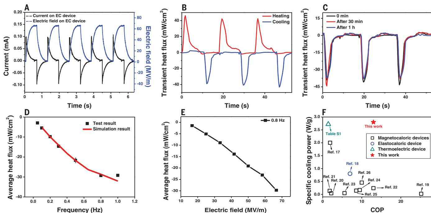
**Fig. 3. Performance of the EC polymer cooling device.** (A) Power consumption of EC film under an applied electric field of 66.7 MV/m. (B) Comparison of heat flux measured by the heat flux sensor in both heating and cooling modes with an applied electric field of 50 MV/m and frequency of 0.06 Hz. (C) Cyclic testing of heat movement transport from the heat source to the EC polymer stack with an applied electric field of 50 MV/m and frequency of 0.06 Hz. (D) Heat flux as a function of different
