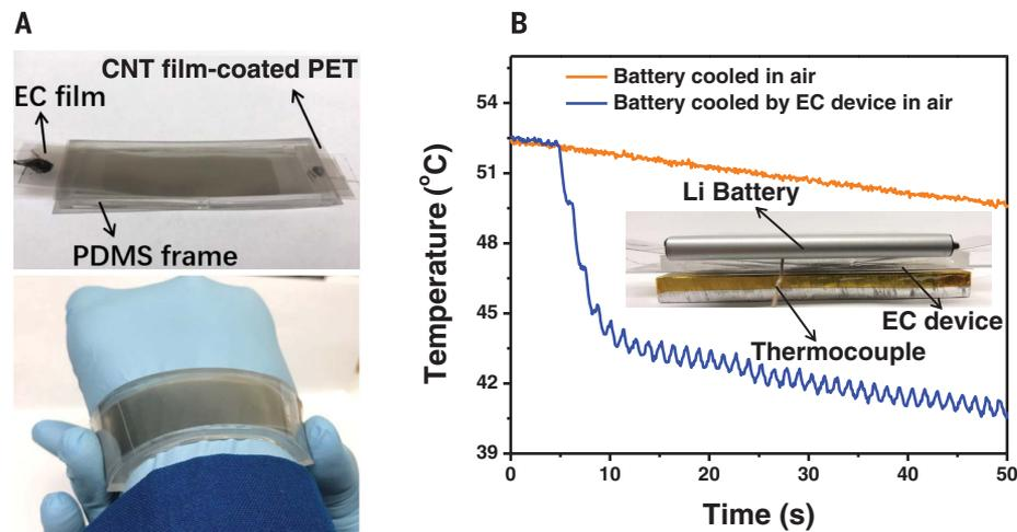
**Fig. 4. Performance of the flexible EC cooling device.** (A) Photograph of a flexible EC device. PDMS, poly(dimethylsiloxane). (B) Temperature change of an overheated smartphone battery with and without an EC cooling device. The inset shows an overheated battery on the top of the EC device.
