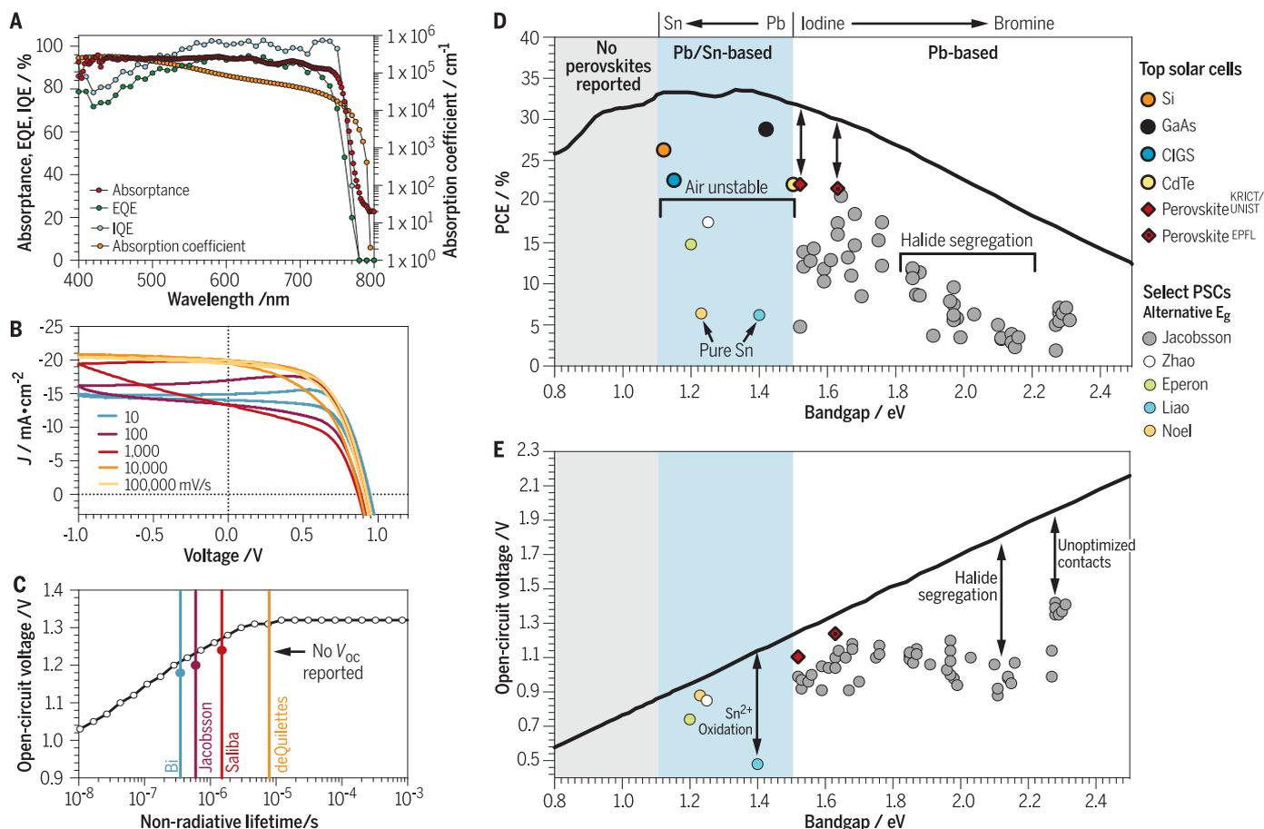
**Fig. 2. Device photophysics of state-of-the-art PSCs.** (A) Light-harvesting efficiency (absorbance), external and internal quantum efficiency (EQE and IQE), and absorption coefficient of a mixed ion-based PSC (14). (B) Current-voltage hysteresis under 1-sun illumination (37). (C) Calculation of the maximum  $V_{OC}$  as a function of nonradiative lifetime for a perovskite layer 500 nm thick, compared with values achieved by Bi *et al.* (18),
