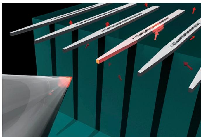
Schematic illustration of silicon waveguides and a YSO crystal
