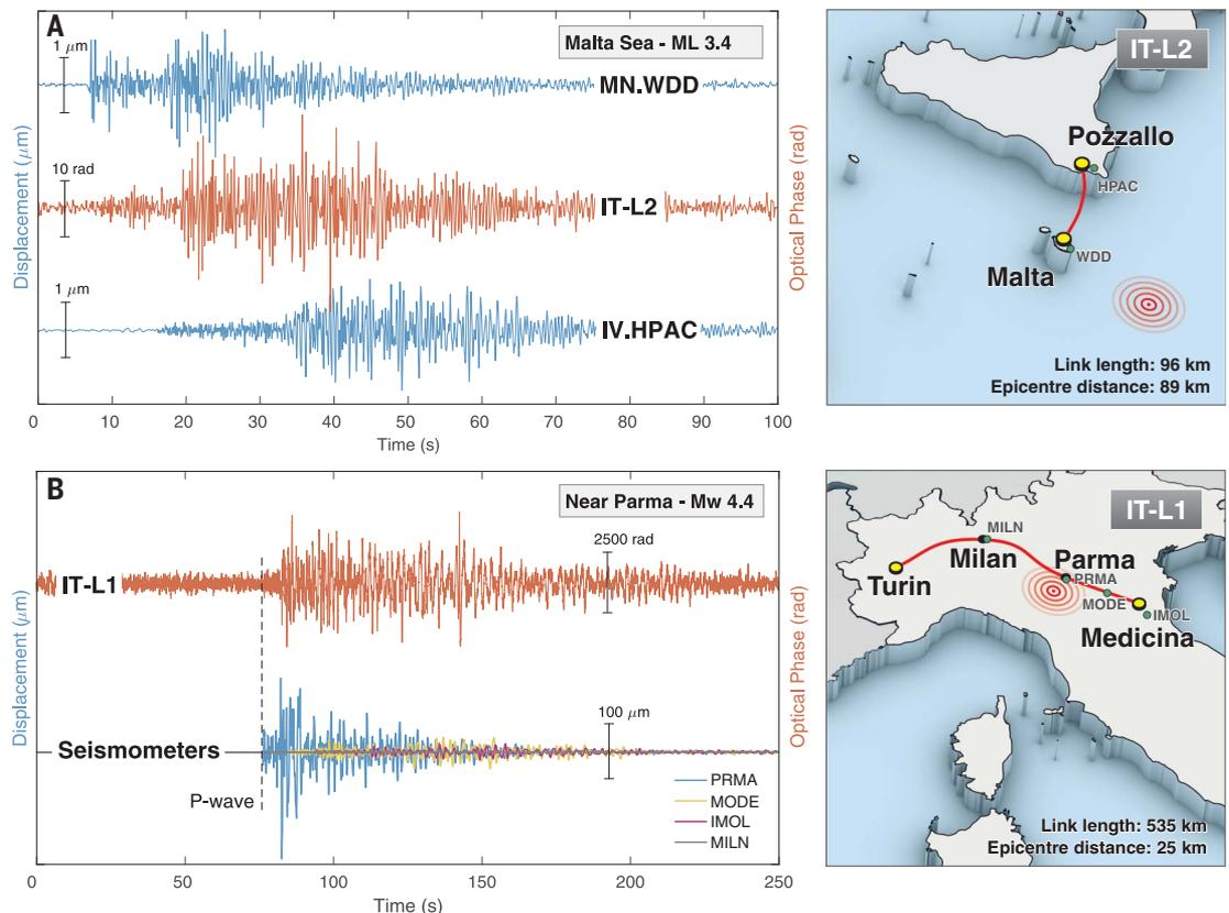
section of the 535-km-long fiber link. We identified the time of arrival of the detected seismic wave, which corresponded to the smallest distance between the epicenter and the fiber link. This also leads to the highest amplitude of the detected signal, as confirmed with the seismometer traces.
