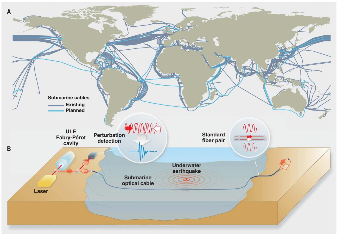
**Fig. 1. Submarine telecommunication infrastructure and earthquake detection experimental setup.** (A) Shown is an illustration of the existing and planned submarine telecommunication infrastructure. Optical frequency metrology techniques enable these fiber links to be used for the detection of earthquakes at the bottom of seas and oceans. [Map data are copyright of OpenStreetMap contributors; cable data are from TeleGeography's
