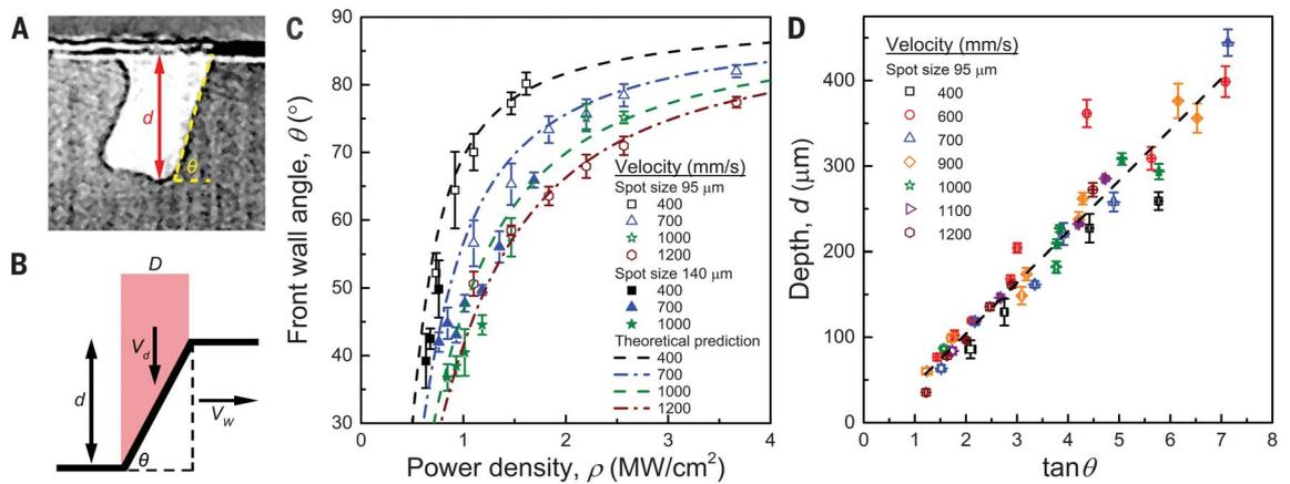
(21). (C) Comparison of the front keyhole wall angles between theoretical predictions (dashed and dash-dotted lines) and experimental measurements (open and solid symbols) for selected beam velocities with spot sizes of 95 and 140  $\mu\text{m}$ . (D) Keyhole depth
