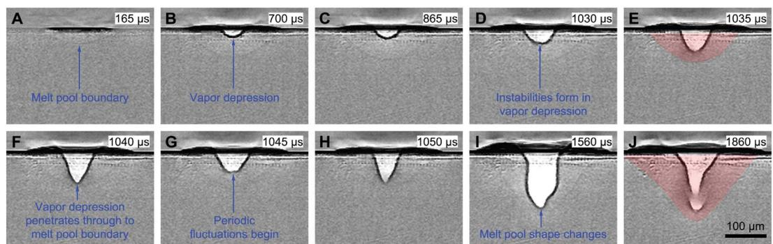
140  $\mu\text{m}$ , and the laser power is 156 W. The images have been background-corrected by the image collected before the laser illumination. The shape of the melt pool is marked with a red shade in (E) and (J).
