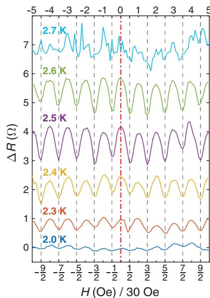
**Fig. 3. Temperature evolution of the Little-Parks effect of the  $\beta$ -Bi<sub>2</sub>Pd ring device.** Oscillations of the resistance as a function of applied magnetic field with the background subtracted for six different values of temperature are shown. The vertical black dashed lines denote the applied magnetic flux of  $\Phi = (n + 1/2)\Phi_0$ . Results are for the same device presented in Fig. 2 (800 nm by 800 nm in area).
