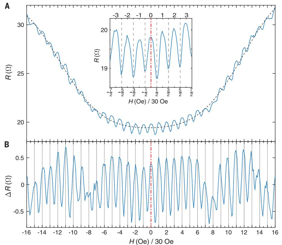
resistance (5). Figure 1E presents a typical result of the Little-Parks experiment obtained from the Nb ring device. The observed oscillation period is 30.2 Oe, in good agreement with 32.3 Oe as expected for  $\Phi_0$  of the 800 nm by
