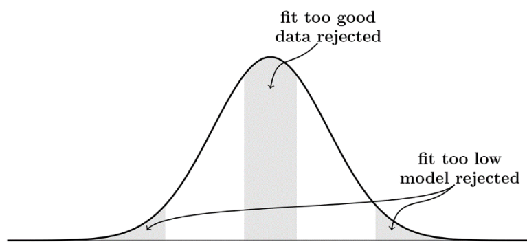
Fig. 6. Thornquist and Crickmore's method of discarding results when data fit prediction doubles the rate of wrong rejection of correct models. Asymptotically, discarding results because data match or mismatch any moment of a predicted distribution raises the rejection rate to 100% of correct models.
