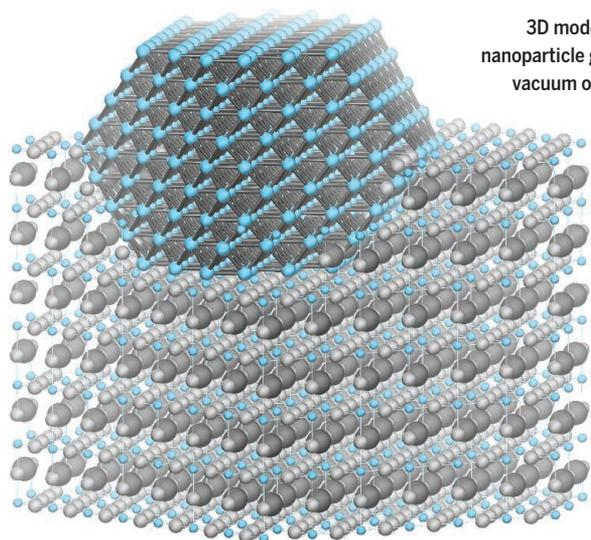
**3D model of a nickel nanoparticle grown under vacuum on perovskite**
