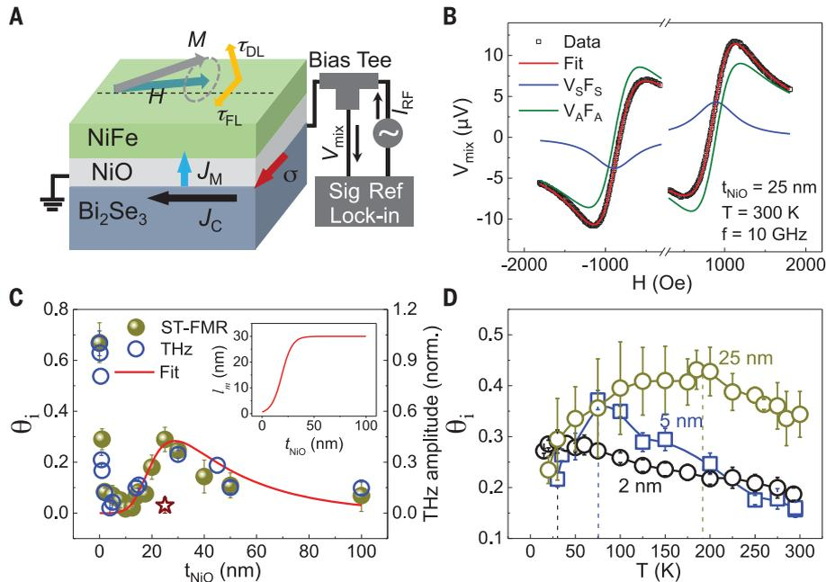
**Fig. 4. Magnetization switching induced by magnon torque in the  $\text{Bi}_2\text{Se}_3/\text{NiO}/\text{Py}$  devices at room temperature.**
