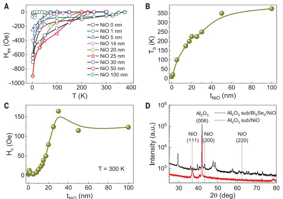
**Fig. 2. Characterization of Bi<sub>2</sub>Se<sub>3</sub>/NiO/Py structures.** (A) The exchange bias as a function of temperature for various NiO thicknesses ( $t_{\text{NiO}}$ ). (B) The blocking temperature deduced from (A). (C) The coercivity as a function of  $t_{\text{NiO}}$  at room temperature. (D) X-ray diffraction patterns of sapphire substrate/Bi<sub>2</sub>Se<sub>3</sub> (8 nm)/NiO (100 nm) and sapphire substrate/NiO (100 nm).
