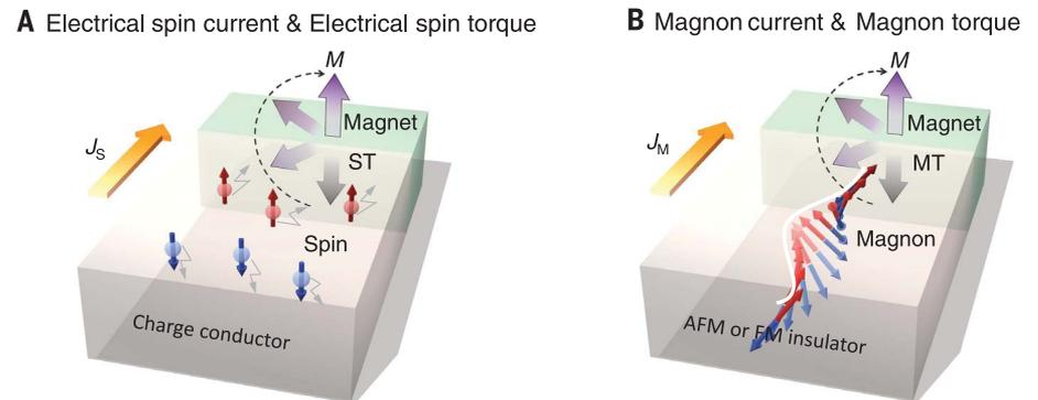
**Fig. 1. Two types of spin-angular-momentum-transfer torque.** (A) Illustration of the magnetization ( $M$ ) reorientation driven by the electrical spin torque (ST) by means of the electrical spin current  $J_S$ . (B) Illustration of the magnetization ( $M$ ) reorientation driven by the magnon torque (MT) by means of the magnon current  $J_M$ . AFM, antiferromagnet; FM, ferromagnet.
