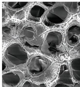
Scanning electron microscopy image showing the macroporous architecture of a bioinspired elastic hydrogel.
