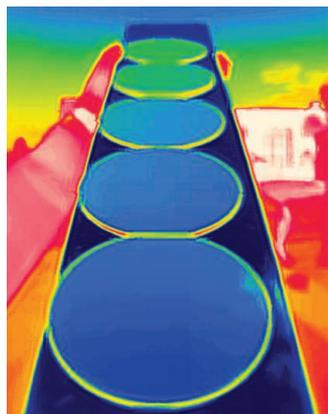
Thermal camera image revealing changes in apparent temperature at different angles for a material with directional emissivity.
