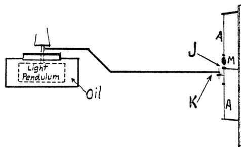
wire *K* attached to the end of an aluminum wire which is itself attached to the light pendulum by a flexible connection. The motion of the pendulum is thus transmitted to the mirror *M* which is cemented to the nickel wire at another point. The rocking of the mirror is recorded in the usual way on bromide paper.
